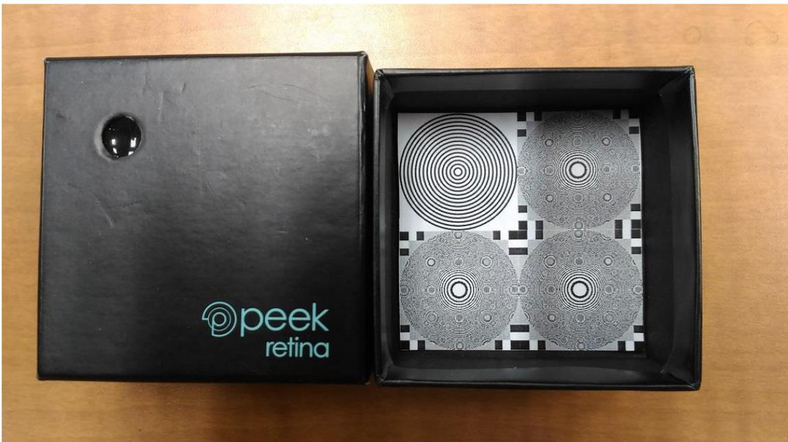
Figure 6. The circular test pattern of the Peek Retina synthetic eye model box
