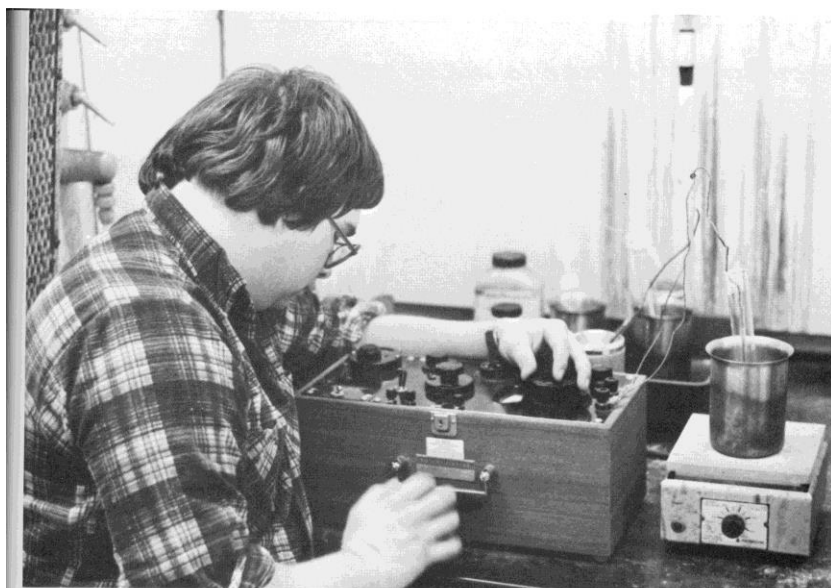
Above: In physical chemistry lab, David Purkiss uses the potentiometer to check the composition of a metal alloy. Left: Slaton Fry performs the very necessary chore of cleaning lab glassware.
