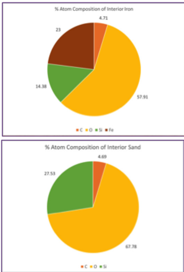
Figure 4. Pie charts of the percent atom composition of two selected areas of artifact R1. The chart on the top is from the yellow circle, and the chart on the bottom is from the blue circle as shown in Figure 3.
