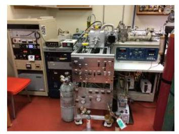
drift cell can also be used to determine the relative amounts of excited and ground state metal ions using a technique called electronic state chromotography, which distinguishes the different states on the basis of their mobilities in He gas. If carried out in the presence of the reactive neutral, a variation on this technique can be used to determine state-specific products and reaction kinetics.
