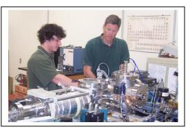
Products of these reactions are then analyzed using a quadrupole mass filter. The drift cell can also be used to determine the relative amounts of excited and ground state metal ions using a technique called electronic state chromotography, which distinguishes the different states on the basis of their mobilities in He. If carried out in the presence of the reactive neutral, a variation on this technique can be used to determine state-specific products and reaction kinetics.
